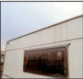
Black streaks may indicate mastic breakdown
